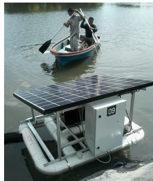
Solar-powered RAPID system for remote monitoring of lake water quality
